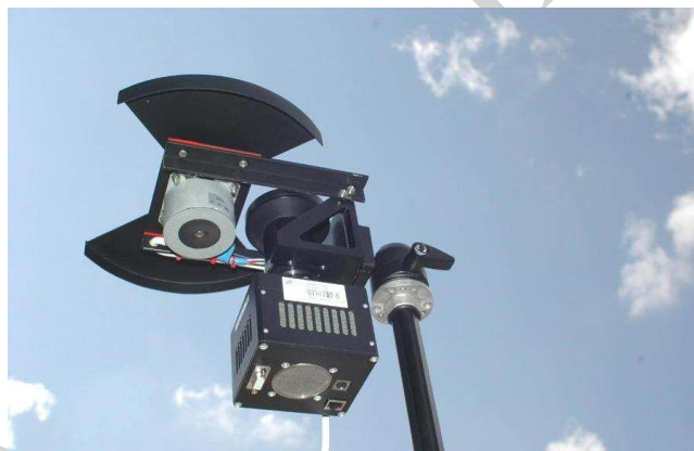
Figure 2 – A SPOSH camera with a rotating shutter at Mt. Parnon.
