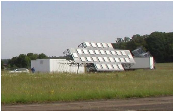
Figure 3 - GRAVES is a bistatic RADAR system.
