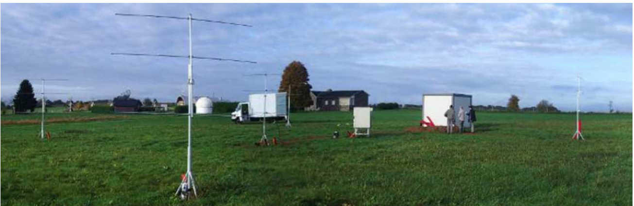
Figure 7 – The BRAMS radio interferometer with 5 Yagi antennas.
