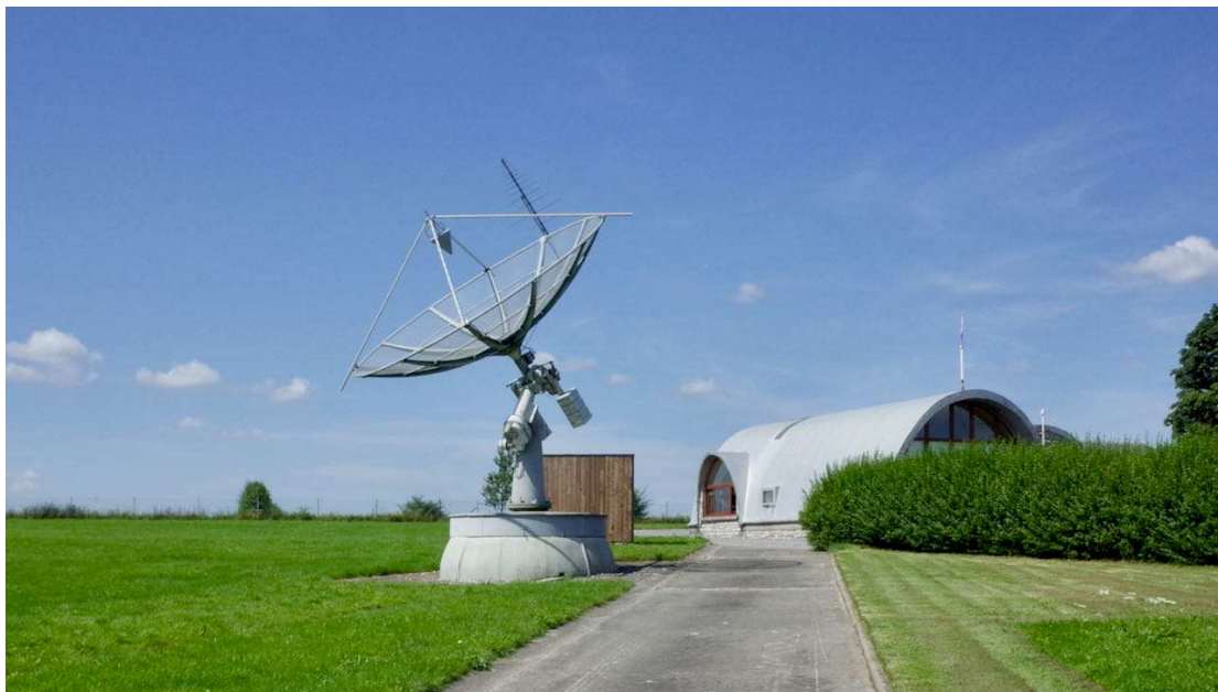
Figure 6 – Antenna refurbished by ROB to track the Sun and take solar radio spectra.
